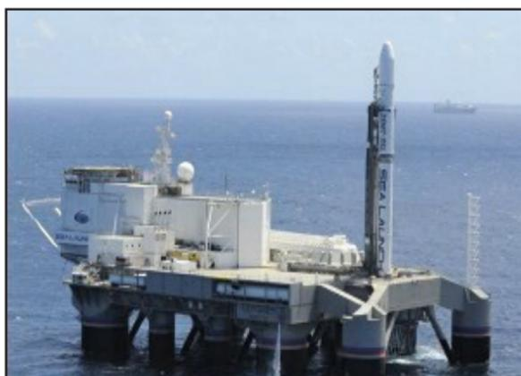
(Photo above) A Boeing-led international partnership modified the drilling platform to launch satellites from near the equator.
